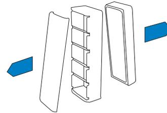
3. Take out the particle filters and carbon filter sheets from each cassette.
