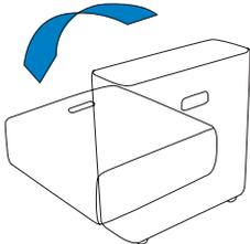
1. Turn off the unit, pull out the power plug, and put the unit down with the backside facing up (on a soft surface like a blanket).
