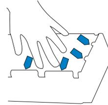
5. Make sure the carbon filter sheets stay in place by pressing down the filters below the tabs on the cassettes.
