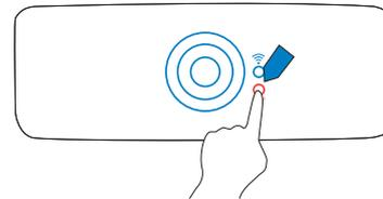
7. Plug in the power cord, put the unit in upright position, and press on the red filter replacement indicator for 10 seconds. Your Sense+ is ready once again to ensure you are breathing cleaner, healthier air.
