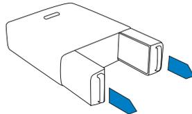
2. Pull out the two filter cassettes using the handles. You may need to pull firmly.
